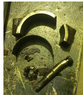
Above : the result of not putting a split pin in a big end bolt....
