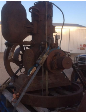
Left : someone used a load binder as a lifting sling.
